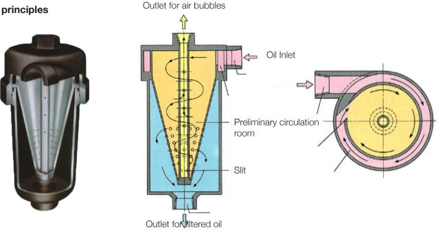
A : Outlet for air bubbles, into the air close to the liquid level
