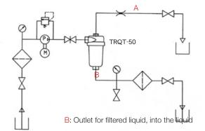
• Adjustment of the flow rate at the Outlet for air bubbles: adjust the flow rate with the Orifice roughly at 5 to 7% of the pump delivery.
